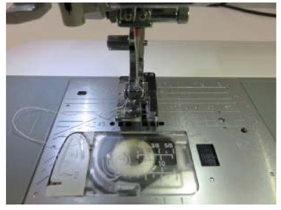
This foot is amazing at keeping seam allowances a consistent 1/4" at all times, by utilizing a little black guide that slides up against the edge of the fabric being sewn.
